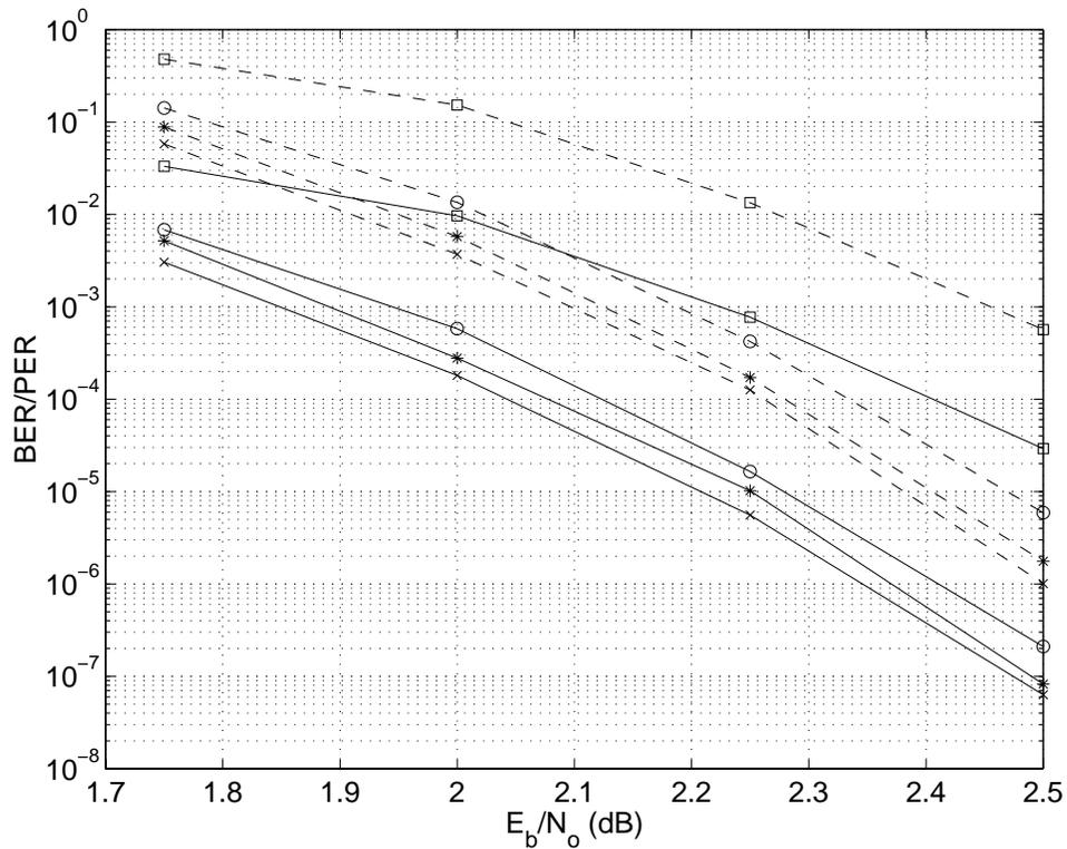
Figure 2: Performance of a (2401,1372) code under True APP (x), optimized scale factor vector (\*), optimized fixed scale factor (o) and standard Max-Log APP ( $\square$ ). Solid line indicates BER, dashed line indicates PER.
