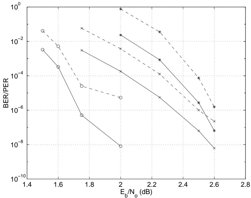
Figure 1: Performance of a various codes under True APP: (2401,1372) code (x) rate  $\approx$  .5801, (14641,10680) code (\*) rate  $\approx$  .7295, (16807,9750) code (o) rate  $\approx$  .5801. Solid line indicates BER, dashed line indicates PER.
