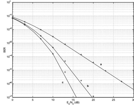
Fig. 1. BER for SC: (a)  $m = 1$ , (b)  $m = 2$ , (c)  $m = 3$ .
