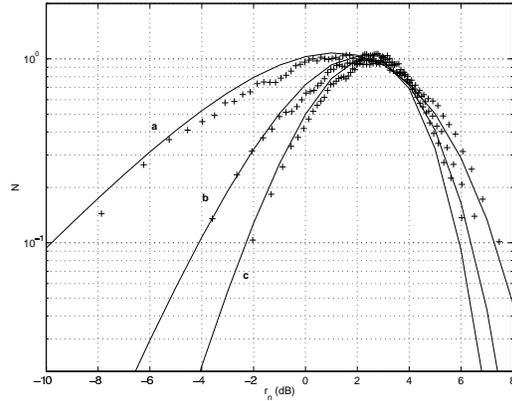
Fig. 6. LCR for EGC: (a)  $m = 1$ , (b)  $m = 2$ , (c)  $m = 3$ .
