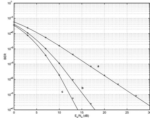
Fig. 2. BER for MRC: (a)  $m = 1$ , (b)  $m = 2$ , (c)  $m = 3$ .
