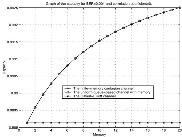
Figure 1: Capacity vs.  $K$  for  $BER=0.001$  and  $Cor=0.1$ .
