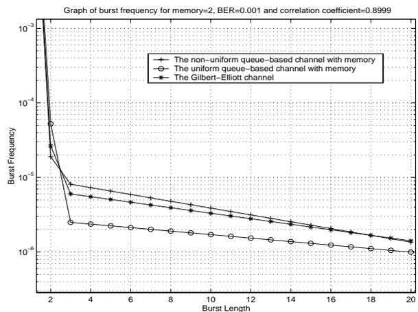
Figure 6: Burst frequency vs. burst length for  $K = 2$ ,  $BER=0.001$  and  $Cor=0.8999$ .
