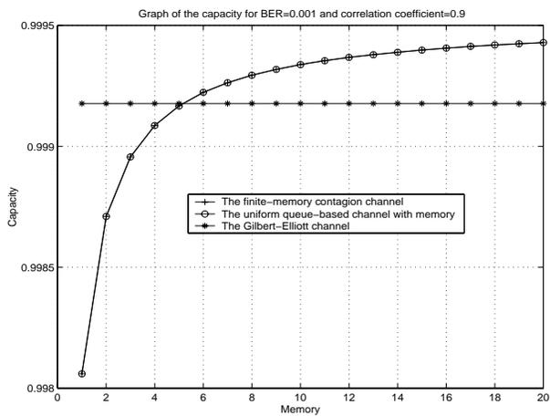
Figure 2: Capacity vs.  $K$  for  $BER=0.001$  and  $Cor=0.9$ .
