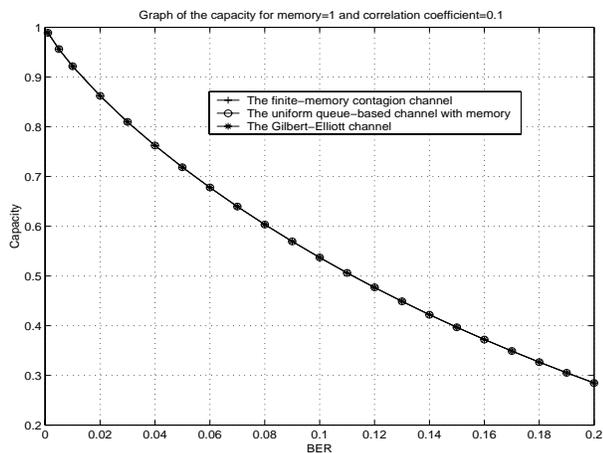
Figure 3: Capacity vs.  $BER$  for  $K = 1$  and  $Cor=0.1$ .
