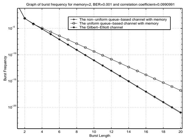
Figure 5: Burst frequency vs. burst length for  $K = 2$ ,  $BER=0.001$  and  $Cor=0.0990991$ .
